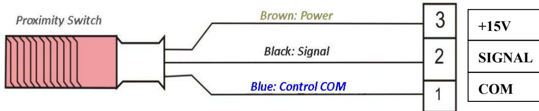
Fig 3-2 NPN proximity switch connection
